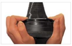
**2.3** Squeeze the two rings together, make sure that the seal does not slide out of its position.
