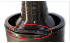
**2.4** if the seal slips out of its groove, it will almost certainly be squashed between the rings. If this happens, detach and restart from image 1.1 (check seal from damage).
