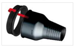
**1.1** Assemble the seal by inserting it through the Oval Stiff Ring, and bringing it back 1,5 cm over the ring.
