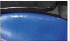
**4.4** Check for creases on the glove continously when pressing the Glove/Oval Spanner Ring into final position. The glove should be positioned as displayed in this image.
