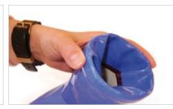
**4.2** Fold the glove shaft inwards over the Oval Spanner Ring, (latex gloves can be fitted and folded the opposite way).
