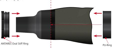
Locate the PU-Ring on the inside of the suit, with its front end positioned at the rear end of the seal. Keep it here while threading the ANTARES Oval Stiff Ring on top of the seal, and finally pressing it into the PU-Ring with the seal pinned in between. Ensure that the Oval Stiff Ring is as close as bottomed into the PU-Ring as possible and that the seal has not been pinned double as this can cause leakage.
