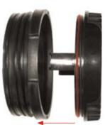
Double O-rings keeps the Oval Glove Ring in place and ensures that the system is not leaking. A latch arm on either side of the Oval Glove Ring engages in a locking groove on each side of the Oval Stiff Ring.
