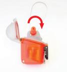
Insert the tool and antenna into the round open space in the back of the top cap.
