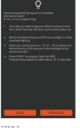
STEP 7 PROGRAM will flash mobile light. GPS will blink white LED twice when successful No further steps necessary
