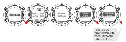
NOTE The settings cannot be activated until 5 minutes has elapsed after the dive.
