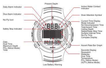
**NOTE**If no button is pressed for 5 minutes, the dive computer beeps and returns to the TIME mode automatically.
