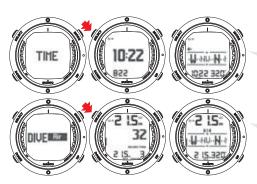
IF ACCESSED FROM TIME MODE, TIME AND BEARING ARE DISPLAYED AT THE BOTTOM OF THE SCREEN.
