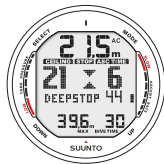
Fig. 6.9 Deepstop. You are advised to make a deepstop at 21m. The second indicator shows that you have 44 seconds left of your deepstop.
