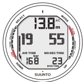
Fig. 6.4 Diving Display. Current tank pressure is 168bar and remaining air time is 19min.
