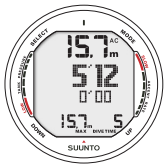
Fig. 6.21. Diving in Gauge mode. Current dive time is 5 minutes 12 seconds.
