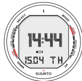
Fig. 5.6. Low Battery Warning. Battery symbol indicates that the battery is low and battery replacement is recommended.
