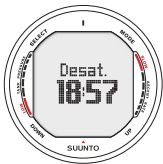
Fig. 7.2. Entering Dive Planning Mode. Desaturation time is displayed
