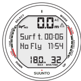
Fig. 6.24. Surface display. It is 6 minutes since you have surfaced from a 32 minute dive, which maximum depth was 18.0 m [60 ft]. The present depth is 0.0 m [0 ft]. Airplane symbol and No-Fly value indicates that you should not fly for 11 hrs 54 minutes. Diver Attention Symbol indicates that you should prolong your surface interval time because of excess micro-bubbles.
