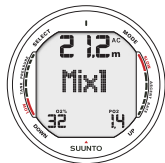
Fig. 6.19 Changing gas mix. Current gas mix is MIX1 (32%). Scroll through enabled mixes by pressing UP or DOWN button. Select new mix by pressing SELECT button.
