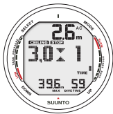
Fig. 6.8. A Mandatory Safety Stop. You are advised to make a one minute Mandatory Safety Stop in the depth zone between 6 m and 3 m [20 ft and 10 ft].
