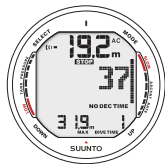
Fig. 6.6. Ascent Rate Indicator. Audible alarm, activated backlight and a blinking full ascent rate bar graph indicate that ascent rate is more than 10 m/min [33 ft/min]. This is a caution to slow down! STOP sign means that you are advised to make a Mandatory Safety Stop when you reach a depth of 6 m [20 ft].
