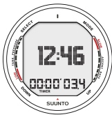
Fig. 3.2. The Stopwatch displays hours, minutes, seconds and tenths of seconds.
