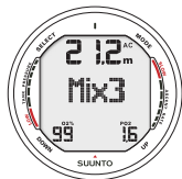
Fig. 6.20 Changing gas mix. Maximum Operating Depth exceeded, gas can not be selected. PO2 value is blinking.
