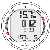
Fig. 6.22. Dive Timer has been reset. Last leg was 5min 23s. You are 12s into current leg.
