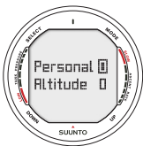
Fig. 5.16. Setting Personal and Altitude adjustment. Press scroll buttons to change personal mode. Use SELECT to accept.
