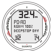
Fig. 6.15. Nitrox Dive Mode Activation. Maximum Operational Depth based on set O_2\% (32%) and PO_2 (1.4 bar) is 32.4m].
