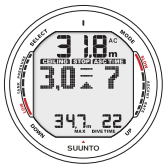
Fig. 6.10. Decompression dive without deepstops, below floor. Upward pointing arrow, blinking ASC TIME label and an audible alarm tell you to ascend. Minimum total ascent time including safety stop is 7 minutes. Ceiling is at 3 m [10 ft].
