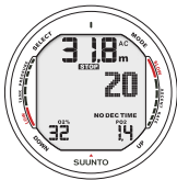
Fig. 6.17. PO 2 Display. Oxygen Partial Pressure is 1.4 bar
