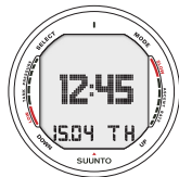
Fig. 2.4. Time mode. Pressing MODE button switches main mode.
