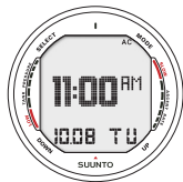
Fig. 2.3. Active water contacts are indicated by the text AC.
