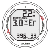
Fig. 6.13. Decompression on dive, above ceiling. Note downward pointing arrow, Er warning and an audible alarm. You should immediately (within 3 minutes) descend to or below ceiling.
