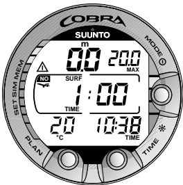
Fig 3.29. Surface interval, Surface time display. Pressing TIME button once will show surface time display.
