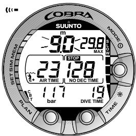
Fig. 3.13. Ascent Rate Indicator. Blinking depth reading, SLOW and four segments are shown together with an audible alarm: ascent rate is more than 10 m/min [33 ft/min]. This is a caution to slow down! STOP sign means that you are advised to make a Mandatory Safety Stop when you reach a depth of 6 m [20 ft].
