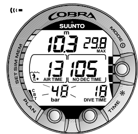
Fig. 3.12. Cylinder pressure warnings. Pressure has dropped below 50 bar [725 psi]. Pressure display is blinking and there is an audible alarm.
