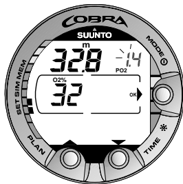
Fig. 4.27. Setting Oxygen Percentage and Partial Pressure. The equivalent maximum depth is displayed as 32.8 m [107 ft]. Press scroll buttons to change oxygen percentage and to set oxygen partial setting value.
