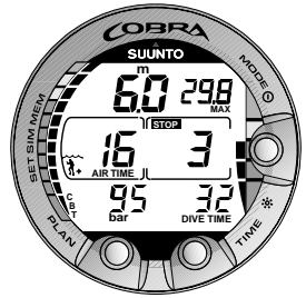
Fig. 3.11. A three minute Recommended Safety Stop.
