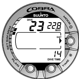
Fig. 4.14. Dive History information. Total number of dives, dive hours and maximum depth.
