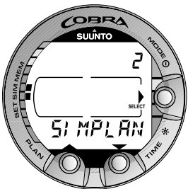
Fig. 4.19. Dive Planning Simulator mode. [2 SIMPLAN].
