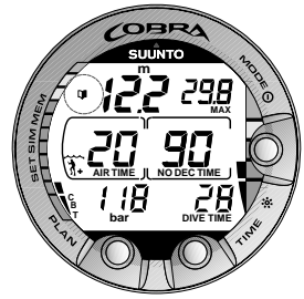
Fig. 3.10. Bookmark activation. An annotation, Bookmark, is placed in the profile memory during a dive by pressing PLAN button. Note Logbook symbol.
