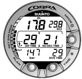
Fig. 3.23. Diving in Nitrox mode. After air time is less than 30 minutes O 2 % is substituted by Air Time display.
