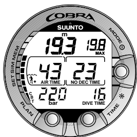
Fig. 3.8. Diving display. Present depth is 19.3 m [63 ft] and no-decompression stop time limit is 23 minutes in A0/P1 mode. Maximum depth during this dive was 19.8 m [65 ft], elapsed dive time is 16 minutes.
