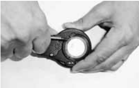
Fig. 5.3. Opening of securing ring.
