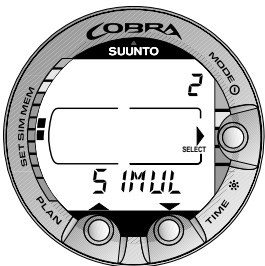
Fig. 4.3. Simulation option. [2 SIMUL].
