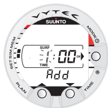
Fig. 4.20. Selected Dive Planning Simulator mode. Add desired surface interval increment (to present shown surface interval) by pressing TIME and PLAN buttons. This display is only shown for repetitive dives.
