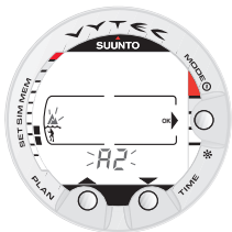
Fig. 4.23. Setting Altitude adjustment. Press scroll buttons to change altitude mode.
