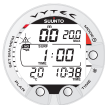
Fig 3.30. Surface interval, Surface time display. Pressing TIME button once will show surface time display.
