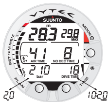
Fig. 3.9. Diving display. Present cylinder pressure is 210 bar [3045 psi] and remaining air time 41 minutes. Alternative display of current time and temperature is shown for 5 seconds after pressing TIME button.
