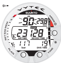
Fig. 3.13. Ascent Rate Indicator. Blinking depth reading, SLOW and four segments are shown together with an audible alarm: ascent rate is more than 10 m/min [33 ft/min]. This is a caution to slow down! STOP sign means that you are advised to make a Mandatory Safety Stop when you reach a depth of 6 m [20 ft].
