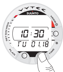
Fig. 2.1. Time keeping display. Pressing PLAN or TIME button activates display.
