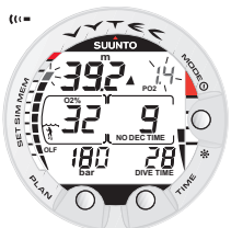
Fig. 3.24. Oxygen partial pressure and OLF displays. There is an audible alarm as oxygen partial pressure is greater than 1.4 bar or set value, and/or the OLF has reached 80% limit.
