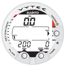
Fig. 4.18. Selected Dive Simulator mode. Descend by pressing the arrow down (TIME) button and ascend by pressing the arrow up (PLAN) button.
