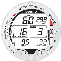
Fig. 3.11. A three minute Recommended Safety Stop.
