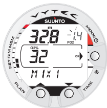
Fig. 4.28. Setting primary gas mix (MIX1). Oxygen percentage is 32%, oxygen partial pressure limit is 1.4 bar. The equivalent maximum depth is displayed as 32.8 m [107 ft]. Press scroll buttons to change oxygen percentage and to set oxygen partial setting value. Accept settings by pressing MODE (OK).
