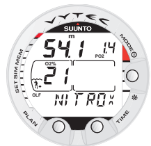
Fig. 3.21. Nitrox display. Maximum depth based on set O 2 % (21%) and PO 2 (1.4 bar) is 54.1 m [177 ft].
